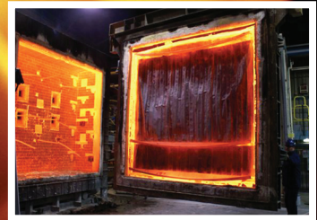
FIREWALL AFTER END OF TEST
